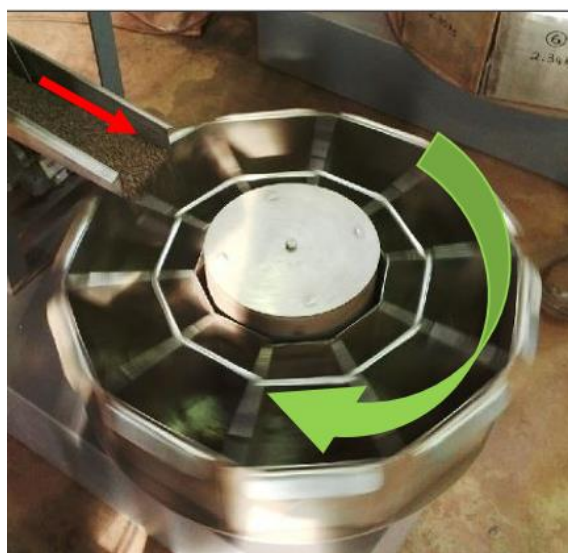
Figure 6. A rotary splitter in operation.
