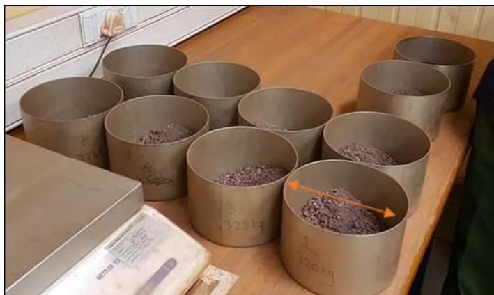
Figure 5. The diameter of the collection cups must not be less than three times the nominal top size of the sample to be split.
