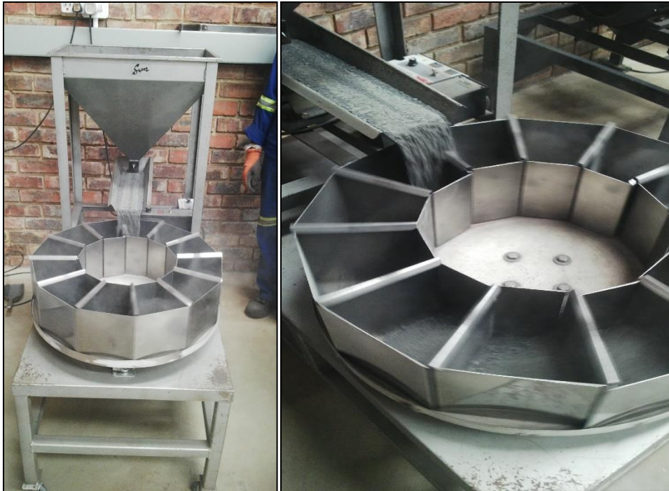
Figure 7. A 12-way rotary splitter. The splitter rests on a durable and level frame.
