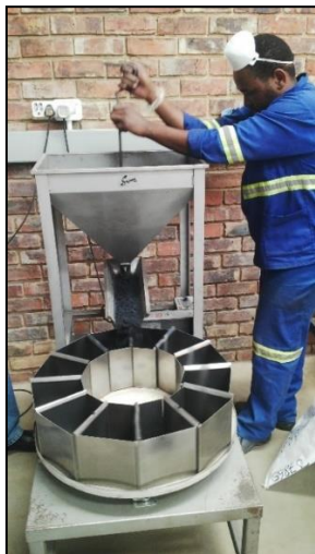
Figure 8. Left: Operator forcing the sample material onto the vibratory feeder. This is not allowed as the sample always needs to be under free flow. Right: The base that the rotary splitter rests on is not level (red arrow), meaning that the splitter itself is not level - this may cause a bias in the splitting of a sample.
