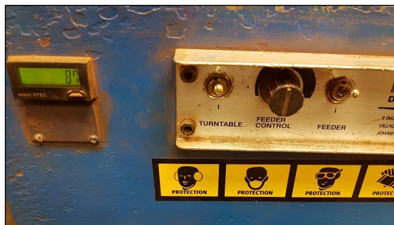
Figure 4. Turntable (carousel) feeder control and feeder switch on a rotary splitter. Some rotary splitters can be field retrofitted with a revolution counter. Here 87 revolutions were recorded to split a sample.
