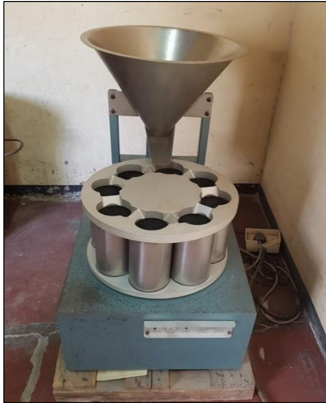
Figure 9. Rotary splitter place onto a wooden pallet. A more stable base is required. Note that the hopper is skew.
